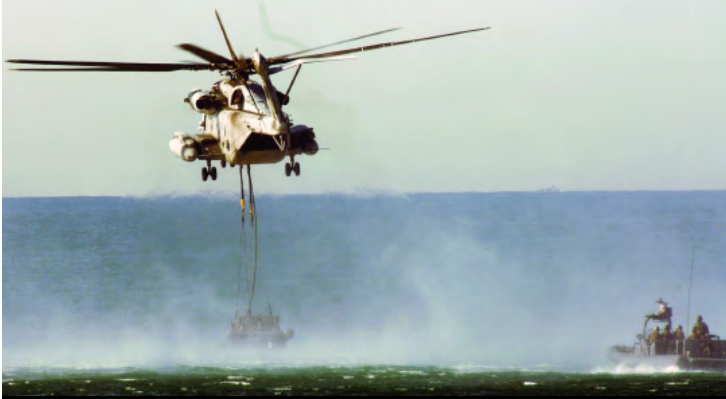
In exercises off the California coast, a CH-53 Sea Stallion heavy-lift helicopter, which the Marine Corps plans to build a new version of, gets ready to release an 11-meter rigid inflatable boat used in special operations.
